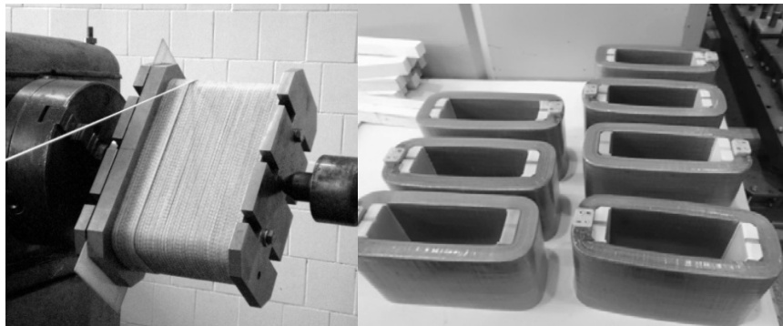
Fig. 4. Winding device and manufactured coils.
