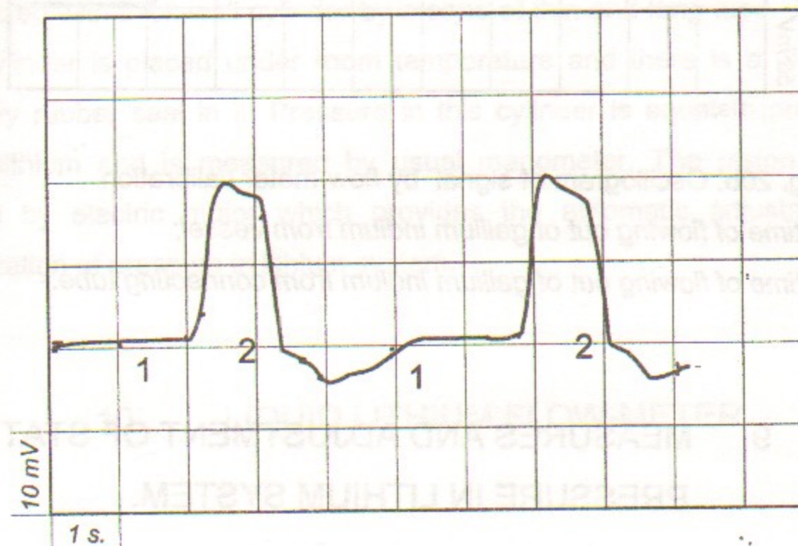
Fig. 20a. Oscillogram of signal from flow-meter by locking valve operation 1-locking valve is open; 2-locking valve is closed. Repetition rate 0.2 Hz.
