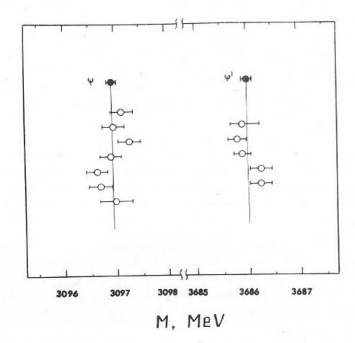
Fig. 2. Results of the Ψ and Ψ'- meson mass measurement at VEPP-4. Open circles - mass values obtained in separate measurement cycles, dark circles - weighted average values.
