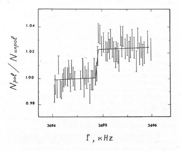
Fig. 1. Experimental values of the normalized counting rate of the particles leaving a beam due to Touschek effect versus a depolarizer frequency. The frequency corresponding to the jump middle is equal to the spin precession frequency of beam electrons.
