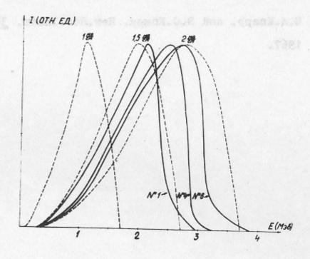
Fig. 3 The spectra of autoemission current (dense lines) and the calculated spectra (dot lines).
