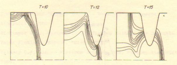
Fig.1 The time pattern of the lines of force of the electric field of a charge traveling past a diaphragm.
