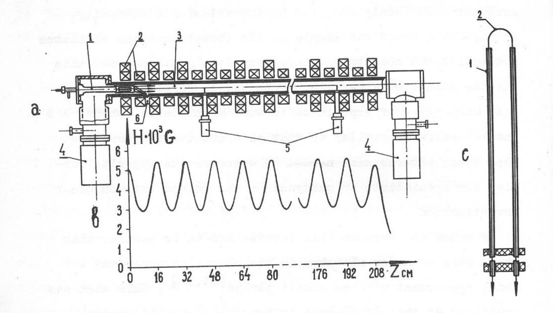
Fig. 3. The model experiment with cesium plasma.
