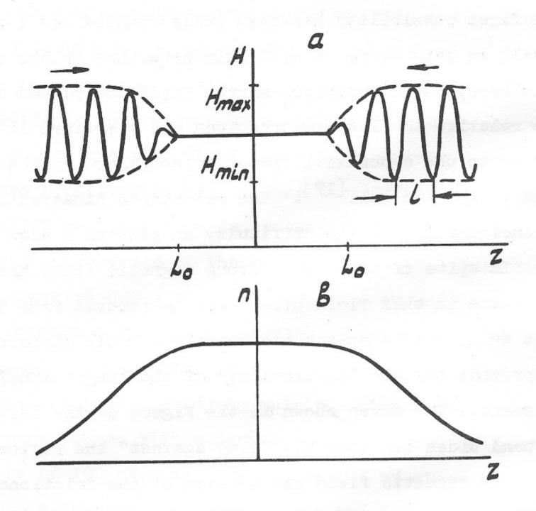
Fig. 5. Stationary confinement of the plasma.
