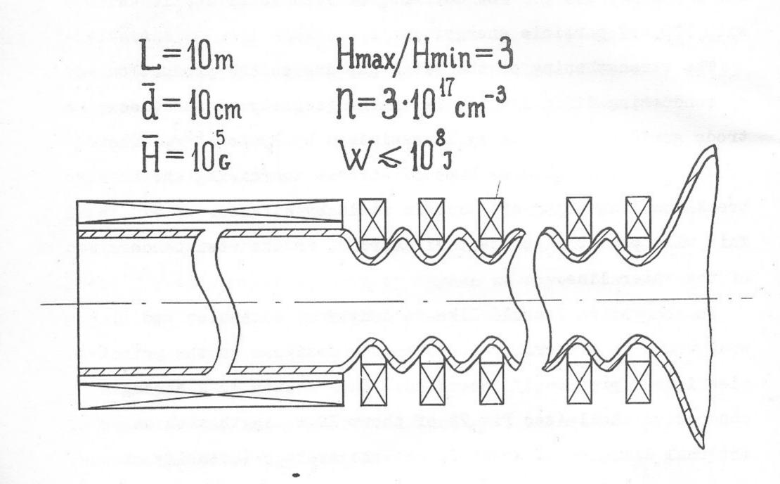
Fig. 7. The diagram of hypothetical thermonuclear reactor with the multiple-mirror magnetic field (Bohm diffusion).
