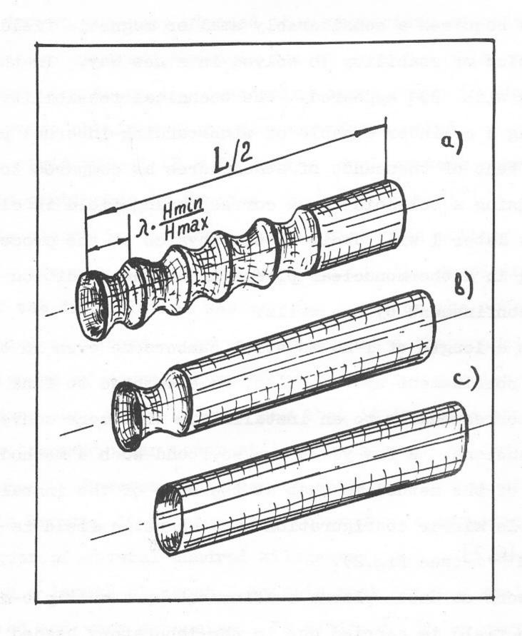
Fig.2. Magnetic surface for: a) corrugated system;
