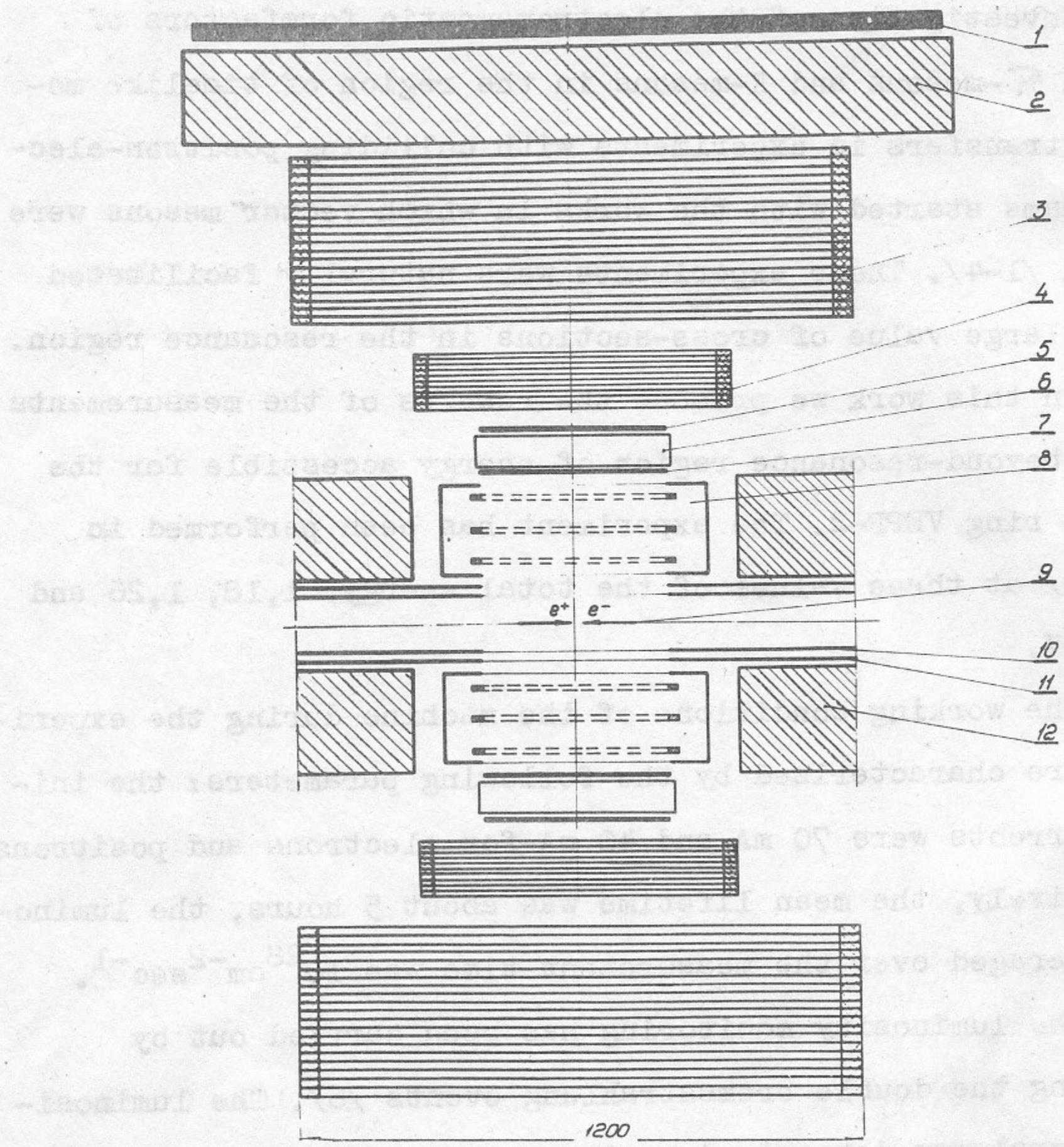
Fig.1. General view of the experimental set-up: 1-anticoincidence scintillation counter; 2-lead; 3-optical "range" spark chamber; 4-optical "shower" spark chamber; 5,7-scintillation counters; 6-water Cerenkov counter; 8-coordinate wire spark chambers; 9-interaction region; 10 and 11-inner and outer vacuum chambers; 12-storage ring magnet.
