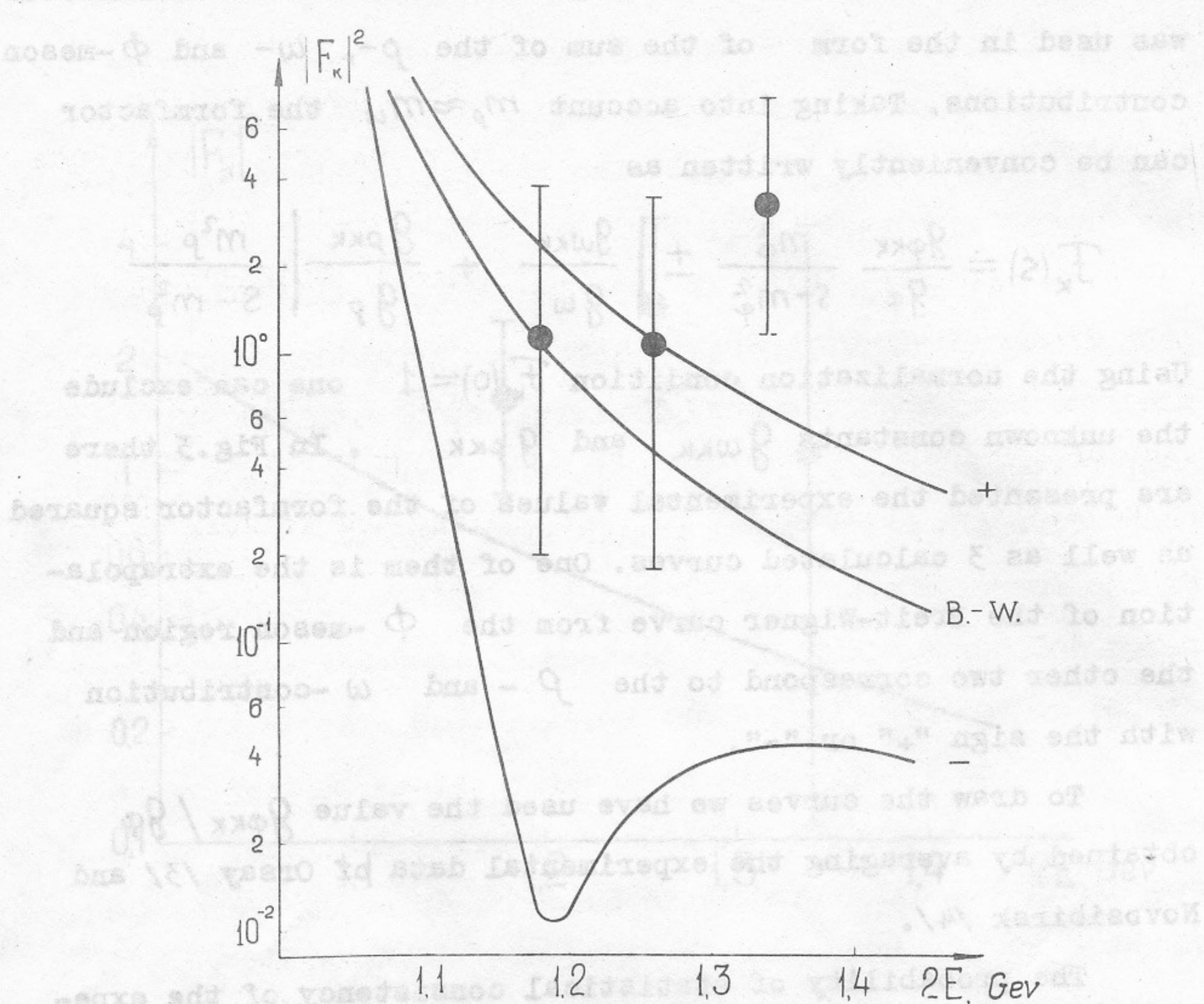
Fig.3. Experimental values of the K-meson formfactor squared. The curve B.W. corresponds to the Breit-Wigner formula extrapolated from the  $\phi$ -meson region. In curves "+" and "-" the contribution of the  $\rho$ - and  $\omega$ -mesons is taken into account with the sign "+" or "-", respectively.
